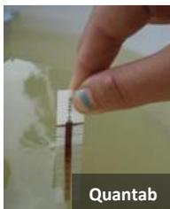
People use different tools to measure salinity. Hydrometers and refractometers are best used in saltier water, while quantabs are best for fresh and slightly salty water.
